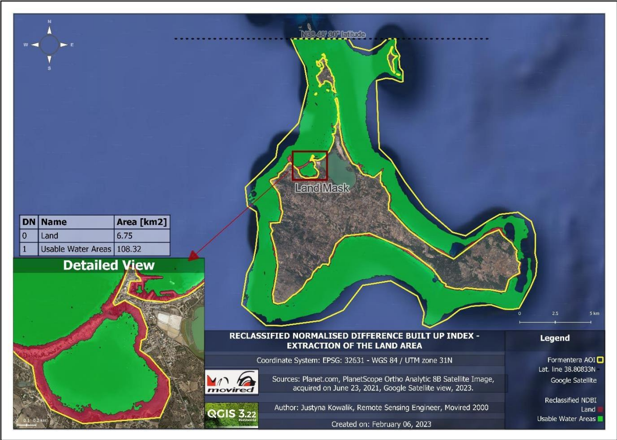
Figure 7. Result of the reclassification of the calculated Normalised Difference Built-Up Index. The unusable areas are marked in red, while the usable, water areas are marked in green.
