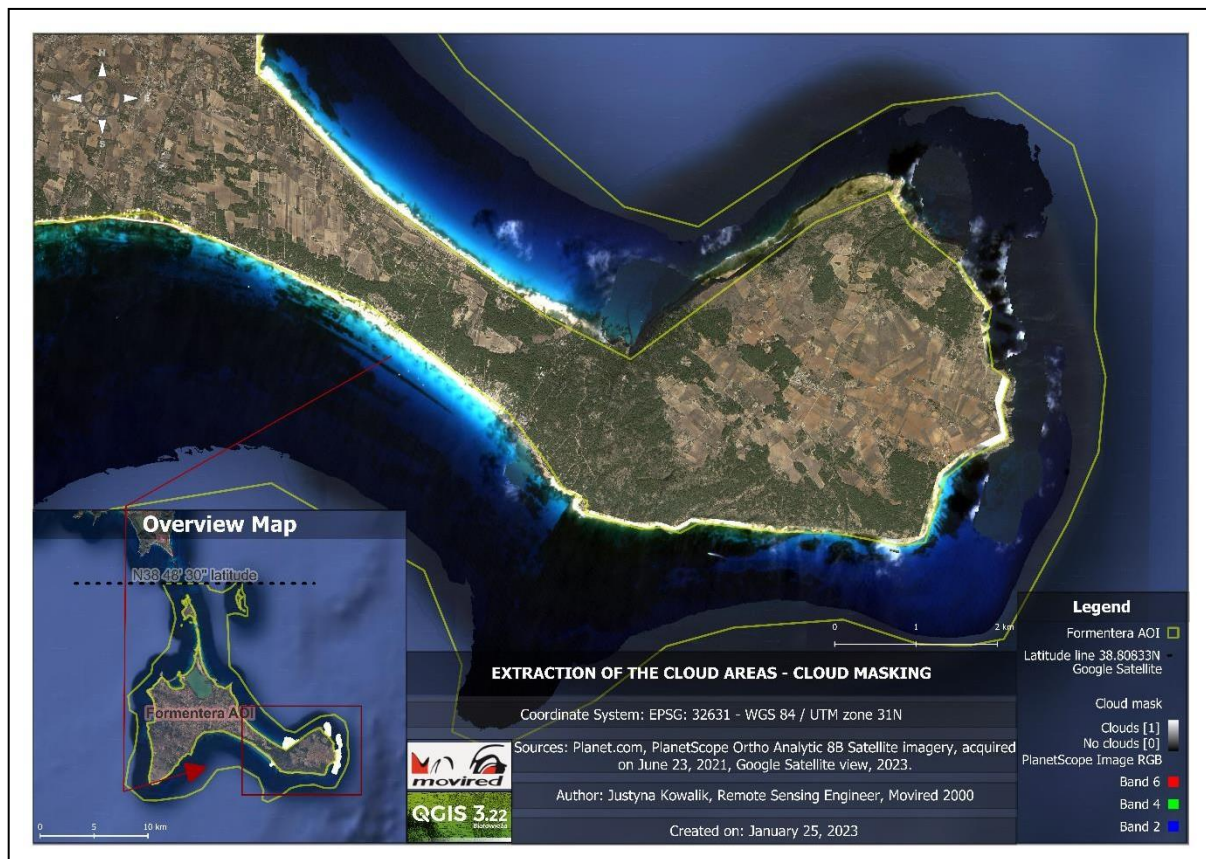
Figure 5. Extraction of the cloud areas (marked in white in the overview map) and the cloud masking of the PlanetScope Satellite image. The cloud areas are clipped out from the image.
