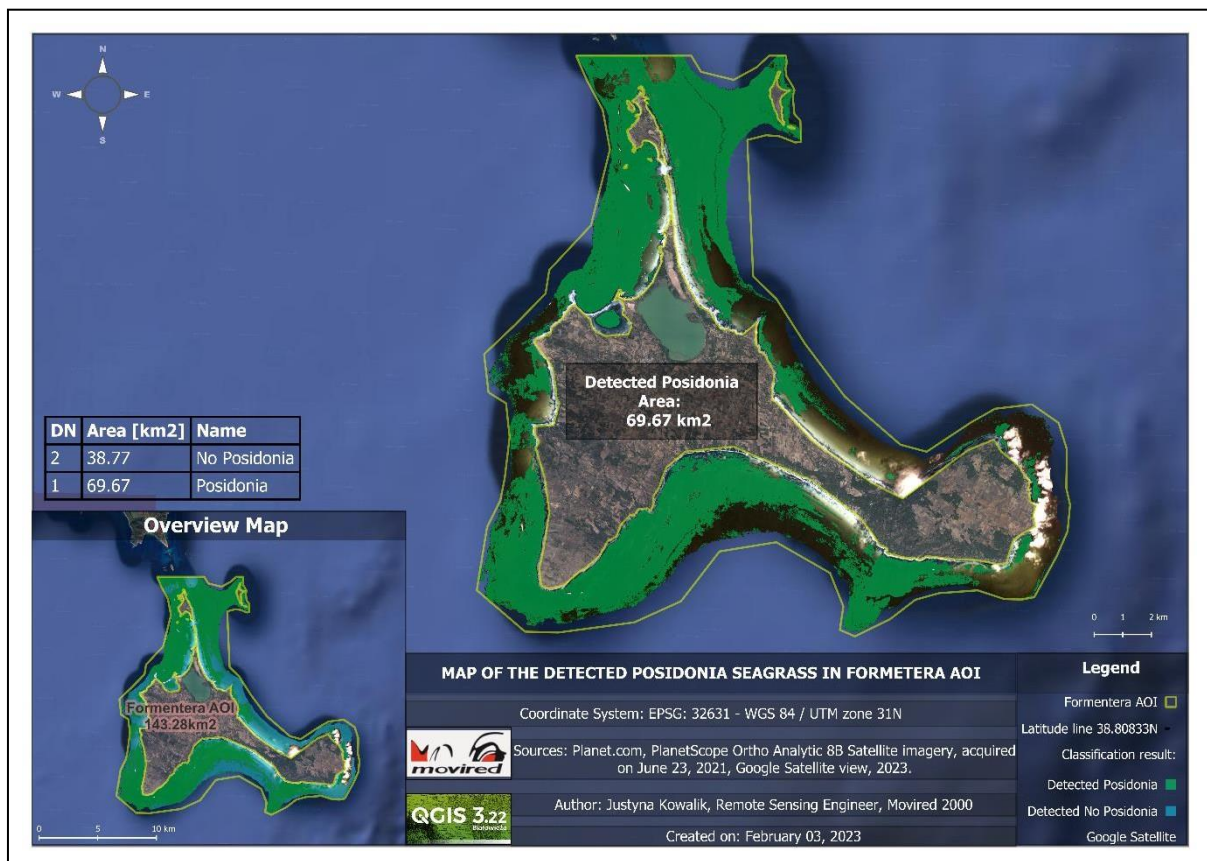
Figure F 1. Vector layer with the detected Posidonia extent is marked in green. The RF classification model predicted the occurrence of Posidonia covering approximately 69.67km 2 .
